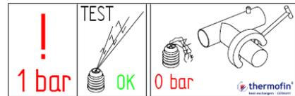
A depressurized device indicates a leakage (Damage in transit!).
