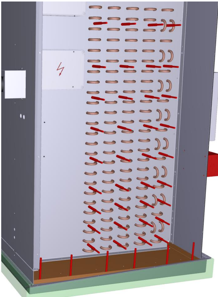
Figure 4: Electric heating rods (red marking)
